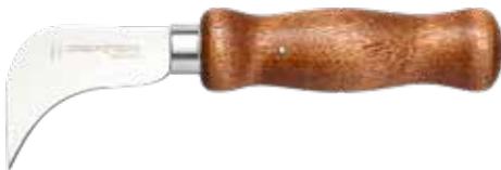
Long Point Linoleum Knife 2 ½" 52160 VX752½ High Carbon Steel, Deep Hook Blade Contour Hardwood Handle with Pin
